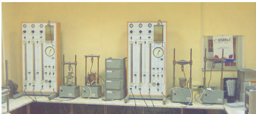
A good laboratory equipped with state-of-the-art triaxial cells is a necessary condition for high quality site investigation results.
